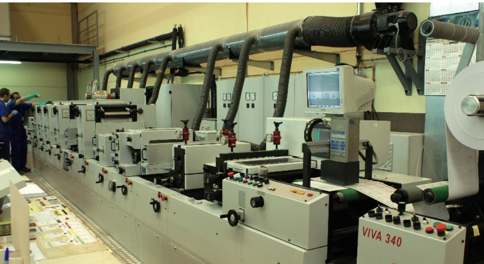
The Codimag Viva 340 5-color waterless offset press at Gràphiques Lappi Martorell in Abrera, near Barcelona
