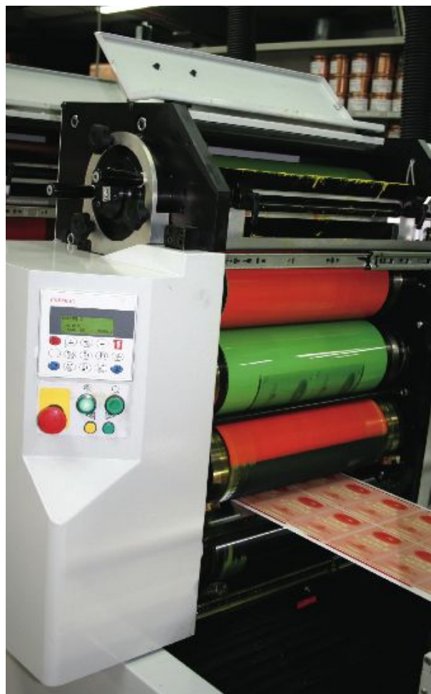
Aniflo uses four cylinders of equal size. An anilox roller delivers a constant ink film to a form rubber roller, which transfers ink to the plate and from the plate to the blanket
