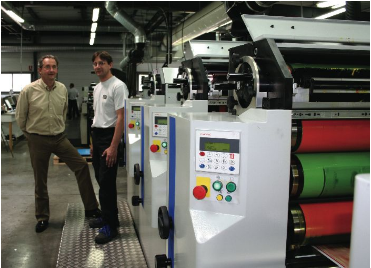
Patrick Wack (left), owner of 5/7 Etiquette, next to the Codimag Aniflo Viva 420 intermittent offset press
